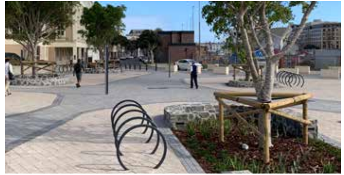
Circular bike racks and seating walls around the tree planter. The tree supplier specified that mature trees should be braced/staked.
